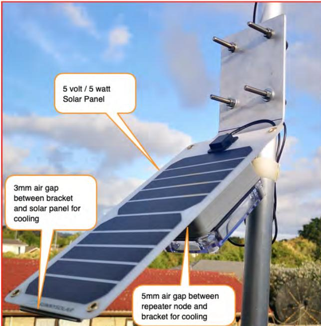
Initial tests showed that heat and humidity were potential issues for the repeater battery and electronics. The repeater now has an internal temperature and humidity sensor with temperature and humidity reported back to the cloud server every hour.
